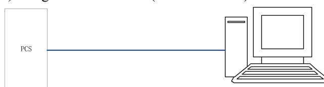
Figure 6.9 Schematic Diagram of Ethernet Communication Solution for a Single Energy Storage Inverter
